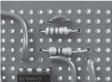
**2l.** Connect one lead of R5 to pin 6 and, using a piece of hookup wire, connect the other lead of R5 to pin 7 of IC1.
