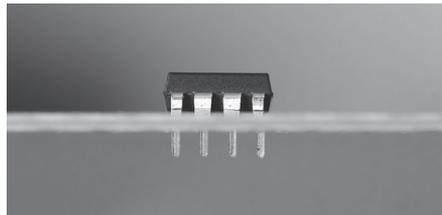
**1e.** Flip the board upside down and fix the chip in place by soldering all eight pins.
