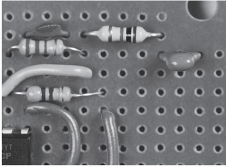
**2n.** Connect one end of R6 to pin 7 of IC1, and the other end of R6 to C3.
