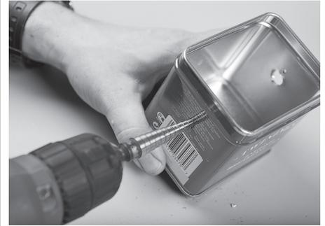
**4b.** Using a power drill, again starting with the smallest bit you have, drill two 1/4” holes into the front of the tin, one for the potentiometer and one for the switch. Switches normally require 1/4” mounting holes, but measure your switch to check. Vacuum the metal shavings out of the tin to ensure that no short circuits occur.
