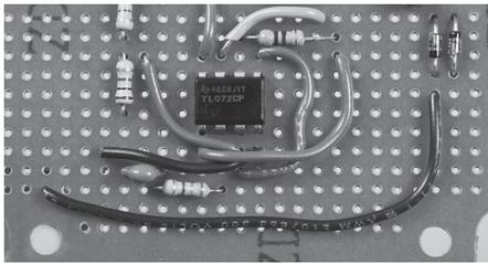
**2q.** Mount C4, noting the polarity of the leads. Connect the negative (-) lead to the circuit ground. Connect the positive (+) lead to the top end of R2.
