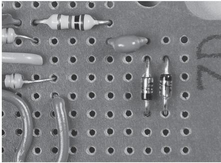
**2p.** Connect the other ends of D1 and D2 together and connect this to the circuit ground.
