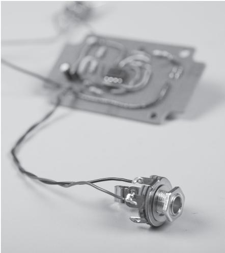
**3f.** Take another pair of different-coloured pieces of stranded hookup wire and twist them together. Connect one wire of this pair to the junction of D1, D2, and C3, and connect same end of the other wire to the circuit ground.
