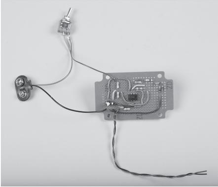
**3e.** Take the free ends of the two wires and connect the one from C1 to the “tip” contact of the input jack, then connect the one from the circuit ground to the ground terminal of the input jack.
