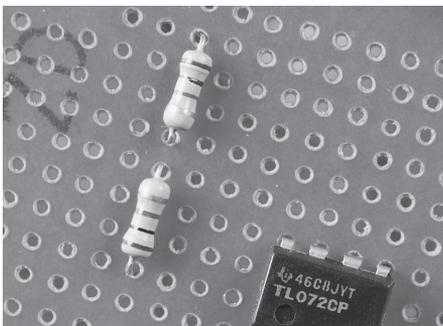
**2d.** Connect the junction of R2 and R3 to pin 3 of IC1.
