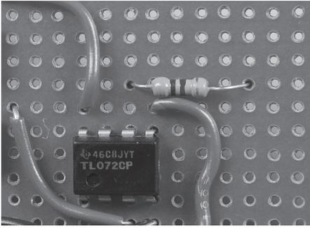
**2j.** Connect one end of R4 to pin 6 of IC1. Then, with a short piece of wire, connect the other end to pin 1.
