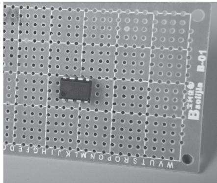
**1d.** You will solder and make connections on the underside of the board, so make sure all the pins of the chip go through the board, and are not bent underneath the chip. Don't force them.
