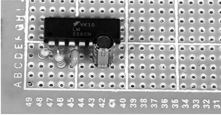
**5e.** Make the pin-to-pin connections on IC4.
