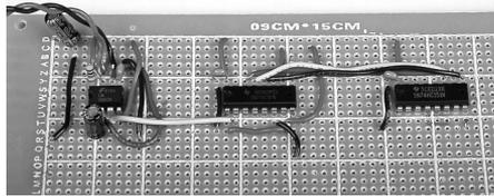
**4g.** Mount R3 and C6 near IC3, and wire them as shown on the schematic:
