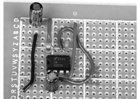
**2d.** Connect to pins 6 and 7 of 555CN chip (IC1) two pieces of stranded wire long enough to reach the potentiometer R1 when the board is installed in the case. It's better to make these slightly long, then trim them in final assembly rather than have them too short.
