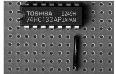
**1g.** Use a short piece of stripped, solid-core hookup wire on the underside of the board to solder a connection between pins 1 and 2 of the chip.
