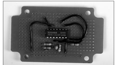
**2h.** Solder resistor R<sub>5</sub> (220Ω) in place and connect one lead to pin 8 of the chip.
