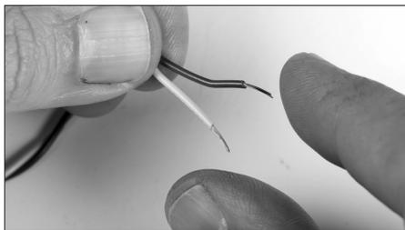
**5d.** Squeeze the stripped end of the second pair of wires, connected in step 4d, and you should hear the tone change. If you don't hear a sound, proceed to the troubleshooting section.
