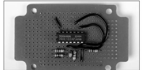
**2g.** Connect the junction of pins 12 and 13 to the negative supply rail. Note that pin 11 does not get connected. Because we're not using the whole chip in this project, we will disable pins 12 and 13 by grounding them.
