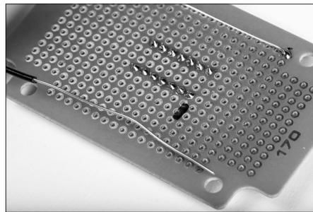
**1e.** Use a length of insulated 22- or 24-gauge solid-core hookup wire, to solder
