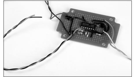
**4d.** Similarly, connect a length of stranded wire to the junction of pins 4 and 5, and R<sub>3</sub> and C<sub>2</sub> (point C on the schematic). Connect another length of stranded wire to the free end of R<sub>4</sub> (point D on the schematic) and twist these two wires together.
