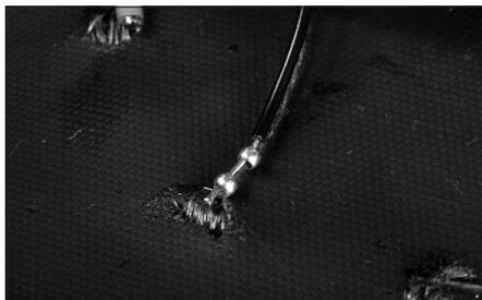
**9g.** Pull the conductive thread so that the circuit wire is taut to the touchpad.
