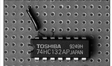
**1f.** As in 1e, solder a connection between pin 7 of the chip and the ground supply rail.
