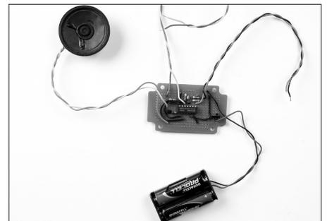
**5b.** Check that the chip is not getting hot (even if you don't hear sound from the speaker!) by touching it carefully, as you would test a hot iron. If the chip is getting hot, immediately turn the circuit off with the switch, remove the batteries, and go to the troubleshooting section of this article.
