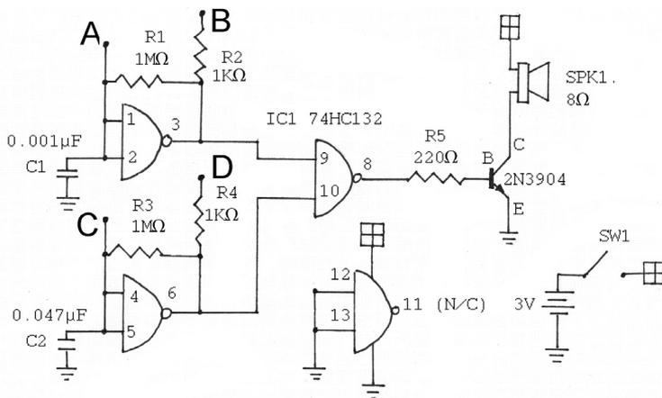
**THE CIRCUIT CONSISTS** of a pair of square-wave oscillators using two of the NAND gates of the 74HC132 chip.
