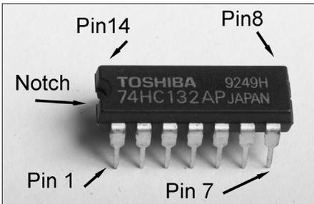
**1b.** Straighten the pins of the chip, ensuring that they're at right angles by slightly bending them on a flat surface, as shown.
