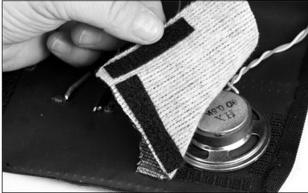
**10d.** Repeat steps 10a through 10c on the underside of the lower left corner of the bag's top flap. This will be a pocket for the circuit's battery holder.
