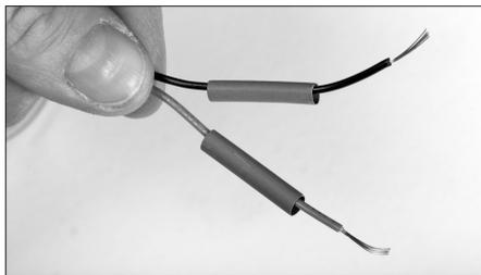
**9d.** Thread two crimping beads onto the wire.
