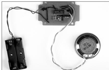
**4c.** Solder a length of 6-inch 24-gauge stranded wire to the junction of pins 1 and 2 of the chip and R<sub>1</sub> and C<sub>1</sub> (point A on the schematic). Solder another length to the free end of R<sub>2</sub> (point B on the schematic), and twist these two wires together.
