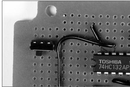
**3d.** If your switch has three terminals (as has the one shown), solder the red lead of the battery holder to the middle terminal of the switch. If the switch has only two terminals, solder the red lead to the free terminal. **NOTE:** Do not install the batteries in the holder at this time.
