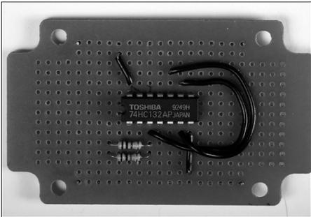
**2c.** Solder resistor R3 (1M $\Omega$ ) in place and connect one lead to pins 4 and 5, and the other lead to pin 6.
