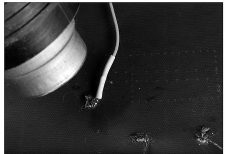
**9k.** Repeating steps 9b through 9j, attach the remaining three circuit leads to the remaining touchpads.
