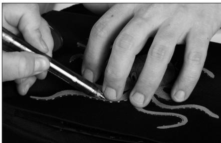
**8b.** Cut a 12-inch piece of conductive thread, thread it through the embroidery needle, and knot one end.
