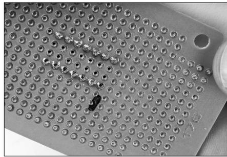
**1d.** Use two pieces of bare wire to establish two power supply rails on the board, one for the ground supply, and one for the positive supply. Some circuit boards come with these pre-made in the copper pattern. The image below shows the positive rail soldered, and the negative one in process. NOTE: The ground will connect to the negative (-) side of the battery, and the positive will connect to the positive (+) side of the battery, via a switch. This will be done later, in steps 1e and 1f.
