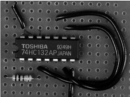
**2b.** Solder resistor R2 (1K $\Omega$ ) in place and, on the underside, connect one lead to pin 3. Leave the other lead disconnected for now.
