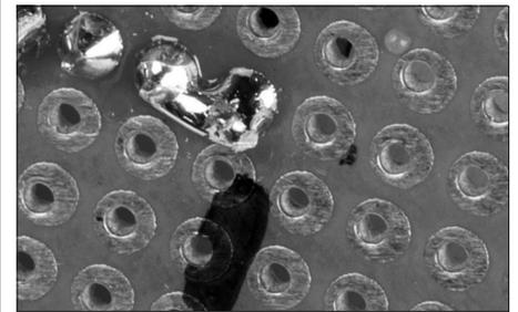
**1h.** As in 1g, solder a connection between pins 4 and 5 of the chip.
