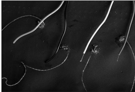
**9b.** Strip a 1-inch length of shielding from one of the circuit leads.
