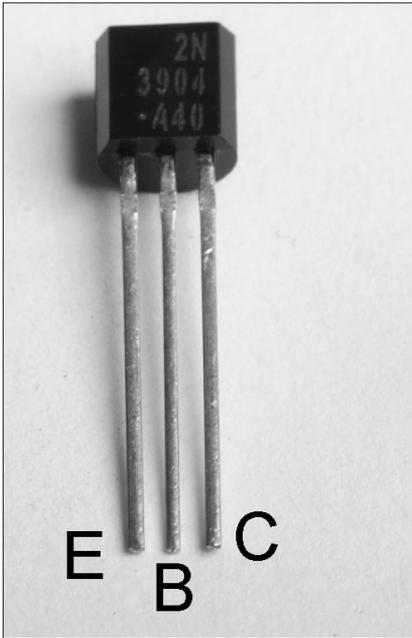
**3b.** Solder the transistor in place, keeping it as close to the board as possible, and on the underside of the board, solder the base lead (B) to the free end of R<sub>5</sub>. Solder the emitter lead (E) to the ground rail with a short piece of insulated hookup wire.
