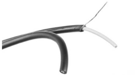
**iii.** Use solder to tin the exposed shield wires.
