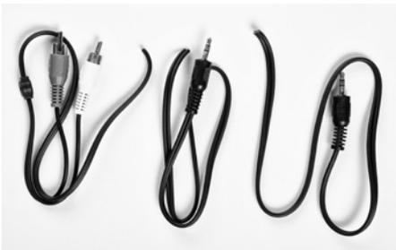
**3b.** Strip and tin the wire ends of the audio cables.
