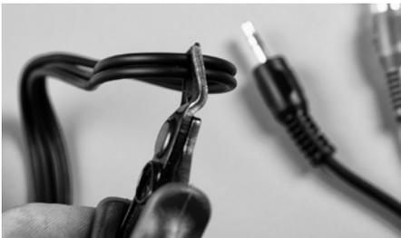
**NOTE:** The two ends with 3.5 mm plugs will connect to the circuit's inputs, and one of the ends with a pair of RCA connectors will connect to the output side. Save the other one for future projects.
