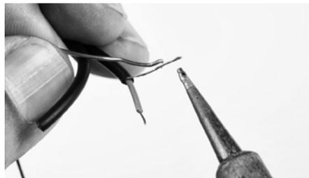
**iv.** Use wire strippers to remove 5 mm of insulation from the centre audio conductor.
