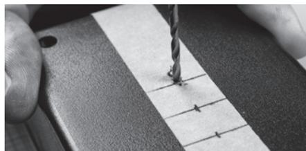
**ii.** Gradually increase the size of your drill bit until the diameter of each hole is slightly larger than the diameter of each photocell. **NOTE:** Don't be tempted to go straight to the largest size, because the drill bit may grab the plastic, ruining the hole, and possibly causing injury.
