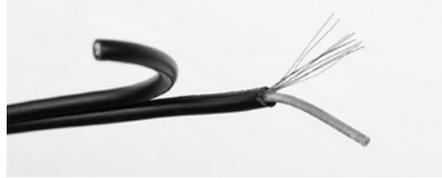
**ii.** Twist together the shield wires.
