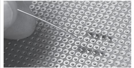
**1f.** Mark pin 1. On the underside of the board, with an indelible marker write 1 to keep the correct orientation when you're working on the circuit board. Note: Because this is a mirror image of the top of the board, the remaining pins are numbered 2 through 8 clockwise around the chip.
