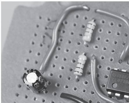
**2r.** Mount C5 connecting the (-) lead to the ground and the (+) lead to the junction of R2 and R3.
