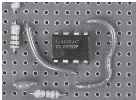
**2f.** Connect a short piece of hookup wire on the underside of the board as shown, from the bottom point of R3. This will be the ground point of this circuit.
