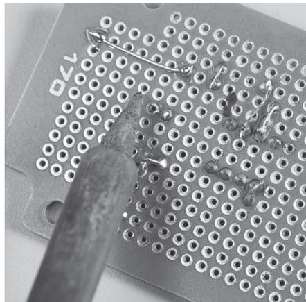
**2g.** Connect the free end of R2 with a short piece of wire to pin 8 of IC1. Note: This is implied, rather than directly shown on the schematic by the "+ in a box" symbol at pin 8. This is not the same as the + symbol at pin 3! (I know; it's confusing.)
