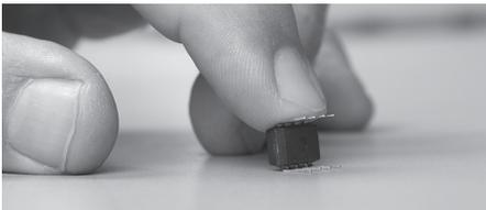
**1c.** Orient the chip on the circuit board, making sure that pin 1 is positioned to the lower left, as shown.
