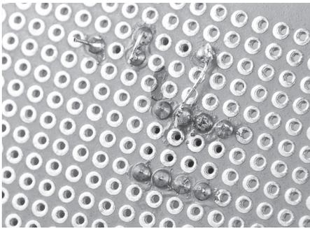
**2c.** Mount R2 and R3 as shown and connect one end of R2 to one end of R3.
