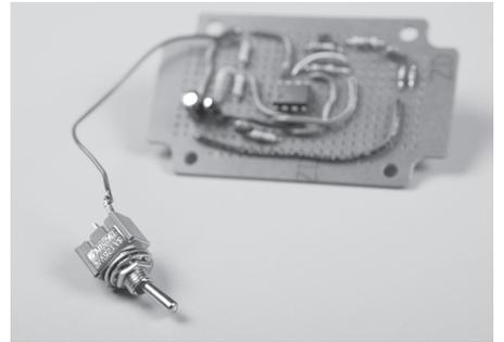
**3b.** Connect the black lead of the 9V battery clip to the circuit ground. Connect the red wire of the 9V battery clip to the free side of the S1 switch.
