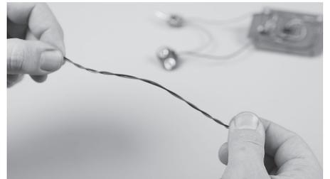
**3d.** Connect one wire of this pair to the free end of C1 and the same end of the other wire to the circuit ground.
