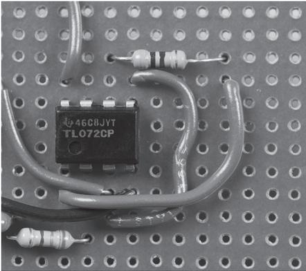
**2k.** Mount C2 and R5 as shown and connect each lead of C2 to the corresponding lead of R5.
