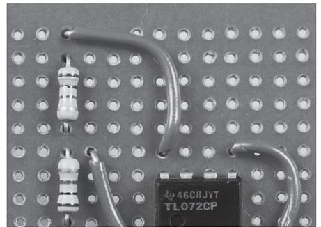
**2h.** Using a short piece of hookup wire, connect pin 4 of IC1 to the common ground point you made previously. Note: This is implied by the "- in a box" symbol at pin 4.
