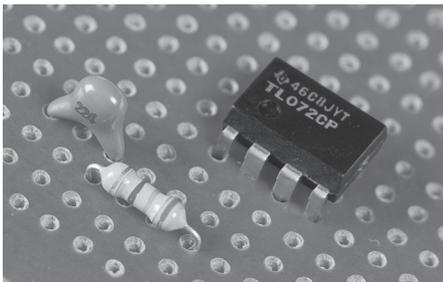
**2b.** Connect one side of C1 to R1, and the other side of R1 to pin 2 of IC1. The other side of C1 will be connected later. Note: Don't get R1, 47k-ohm, mixed up with R4, 4.7k-ohm.
