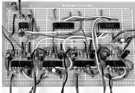
have used multiple supply rails, make sure they are all properly connected.
