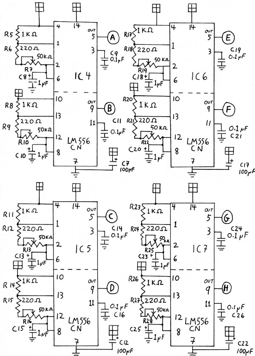
**NOTE:** The connections in the following steps are separated on the schematic, and indicated by the circled letters A (for first oscillator circuit) through H (for eighth oscillator circuit), indicating which outputs of ICs 4, 5, 6, and 7 should connect to which inputs of IC3. Take careful note of the pin numbers on IC3.
