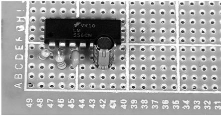
**5e.** Make the pin-to-pin connections on IC4.
